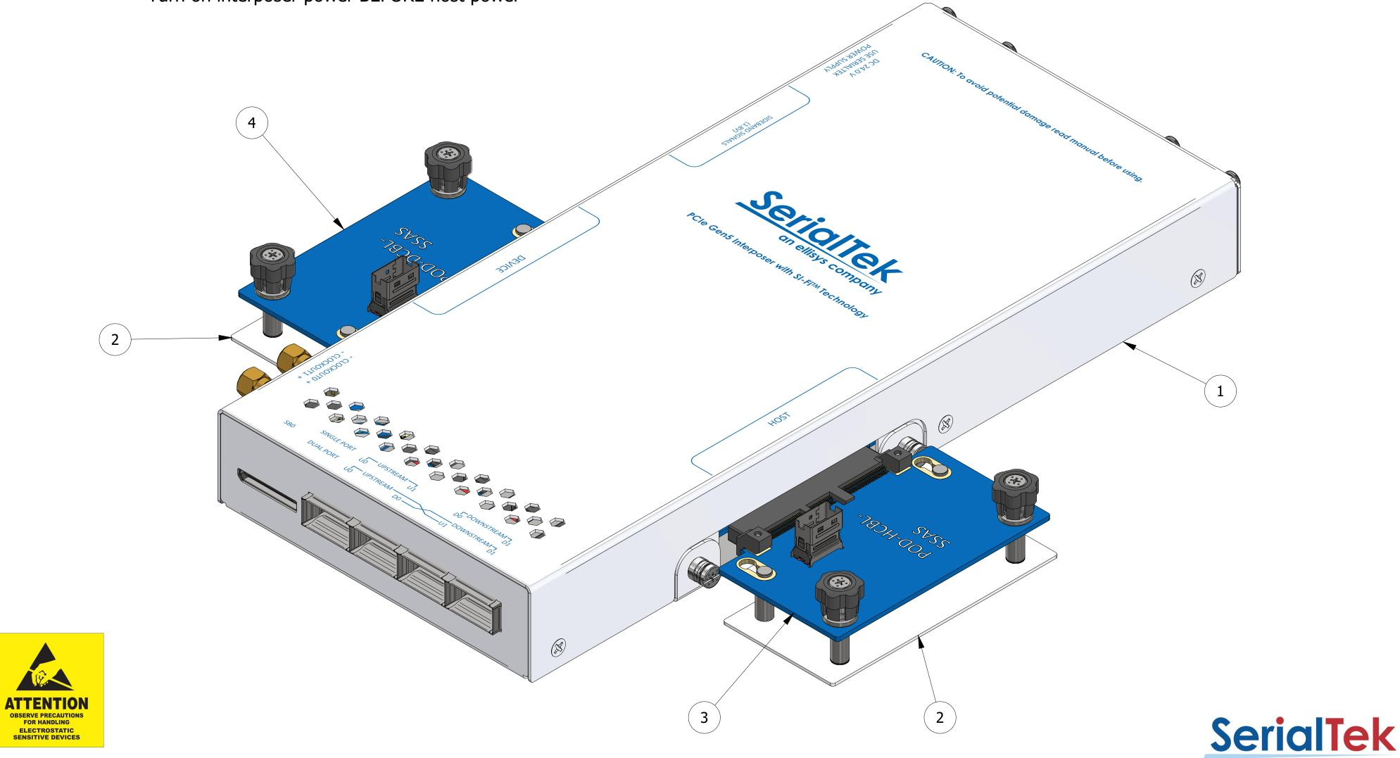
Slide the Host/Device Cable Adaptor Tray into the slot on the DEVICE side on the underside of the POD Main Unit at an angle of about 60°.
