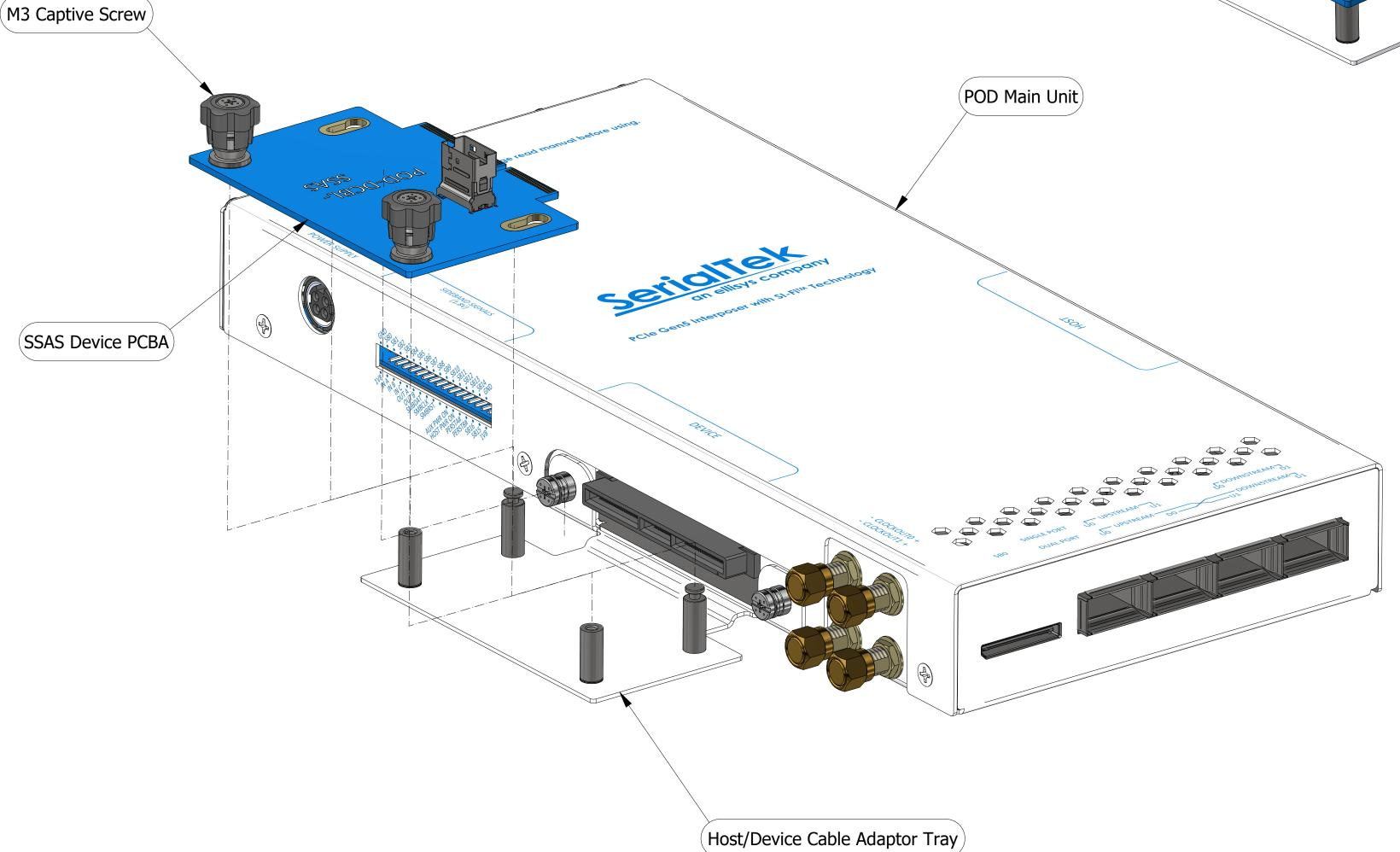
Slide the Host/Device Cable Adaptor Tray into the slot on the HOST side on the underside of the POD Main Unit at an angle of about 60°.
